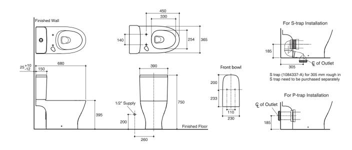
Note: The recommended dimension for installation can be adjusted according to user preferences and layout. Kohler Co. reserves the right to make changes in product characteristics, packaging, or availability at anytime without notice.
